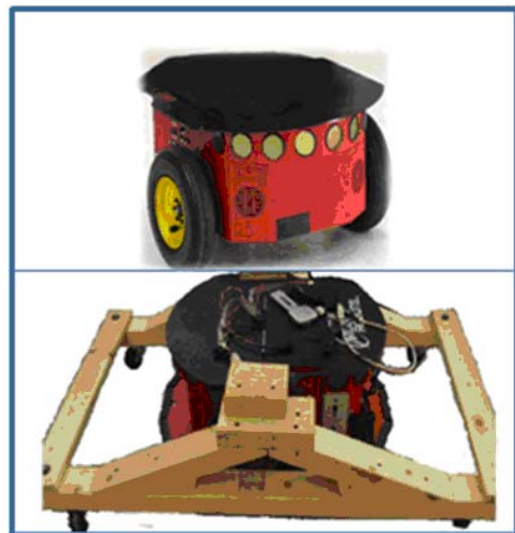
Fig. 2. Starting from the base of the Pioneer 3-DX robot, an extension base was added to improve stability so that a child would stand on the robot.
